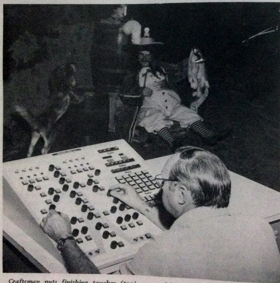
Craftsman puts finishing touches (top) on model depicting Paris street scene in preparation for presentation of World Showcase plans. Operations at WED range from artistic endeavors to such sophisticated engineering problems as programming audio-animatronic figures, as the engineer above is doing at control panel. (Copr. Walt Disney Productions)
