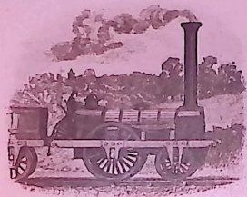
One of the first passenger engines built by George Stephenson, who, in 1816 patented engines that would travel 16 miles an hour—without a load.
