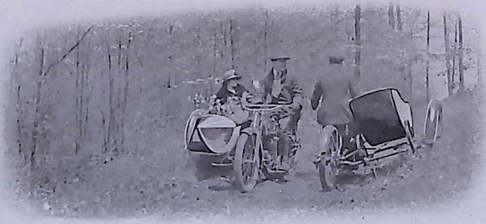
Holiday voyagers passing on a narrow wooded lane--note sidecar wheels running along bank higher than road, without tipping motorcycle over, or making any difference in steering.
