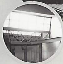
A TUBE MILL. DRAWBENCHES REDUCE THE THICKNESS AND INCREASE THE LENGTH OF TUBES
