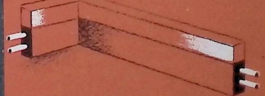
Radiant heating by means of hot water or steam coils concealed in floor or walls
