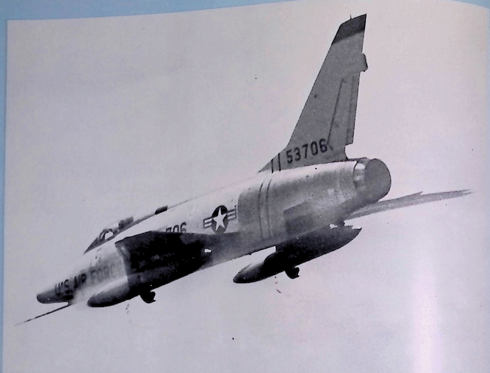
Twin 20mm Vulcan cannon pods (VULPOD) slung under wings of an Air Force F-100 during in-flight test evaluation, together pump out rounds at a rate of 12,000 shots per minute. Spent cartridges can be seen trailing behind the jet aircraft.
