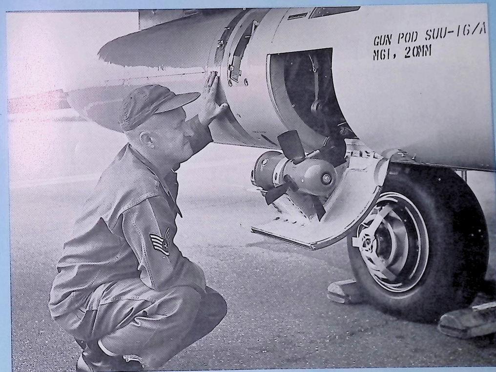
Ram-air turbine automatically extends from VULPOD, 20mm Vulcan cannon in a detachable pod, when pilot prepares for firing run. Turning at a constant 12,000 shots per minute, it transmits power to the gun and feed system, bringing the gun to its 6,000 shots-per-minute firing rate in 0.4 seconds.
