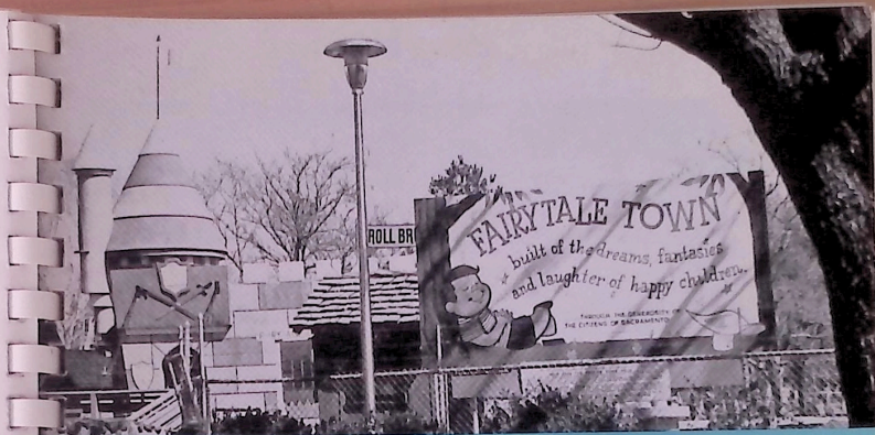
Fairytale Town, in the city park at Sacramento, increases its early evening business by lighting its grounds with L-M PTL's. These light fixtures use only 300 watt lamps spaced 100 feet apart. PTL's glass refractor directs the light down where it is usable.
