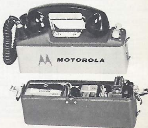
"Snap-On" Power Packs: Standard & Extra-Duty Dry Cell, Rechargeable Nickel-Cadmium-6/12 Volt, Wet Cell, 12/24 Volt, 117 Volts AC, 60 Cycles
