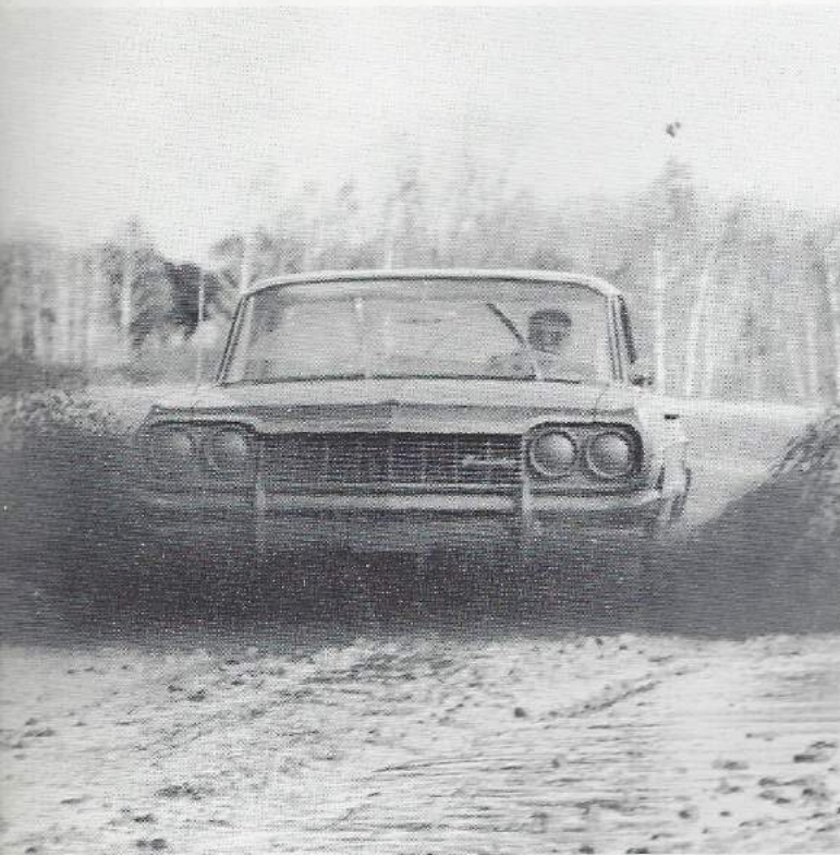
(Left) Mud quagmire and (Right) 1,000-foot bathtub are part of punishing test program GM cars undergo at Milford Proving Ground
