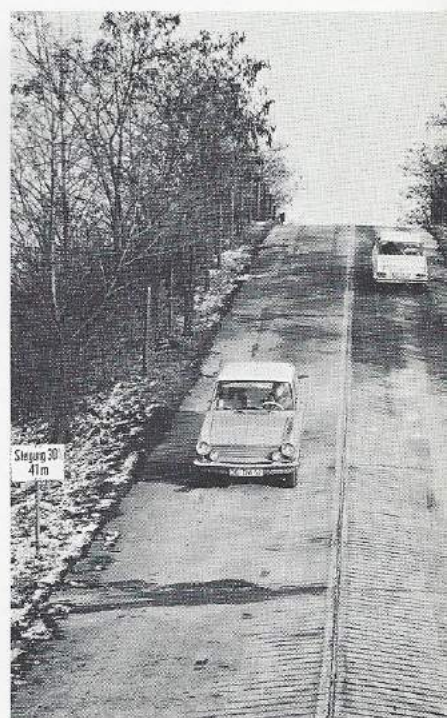
Kadetts are tested on 30% grade at Opel test track in Russelsheim, West Germany
