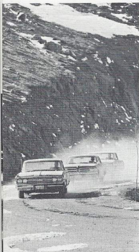
(Above) When 36,000-mile durability run at GM's Milford Proving Ground is completed cars are dismantled for detailed inspection by engineers and designers. (Below) Three GM cars climb to summit of Pikes Peak to test engines and transmissions under extreme grade and altitude conditions
