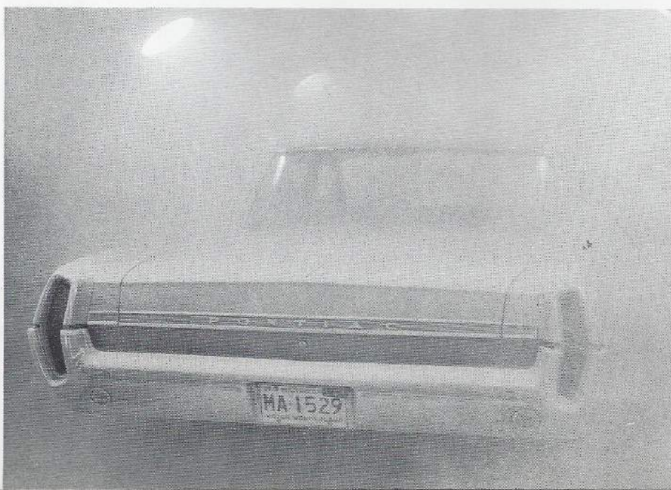
Fisher Body engineers create severe dust storm in laboratory to test door and window seals
