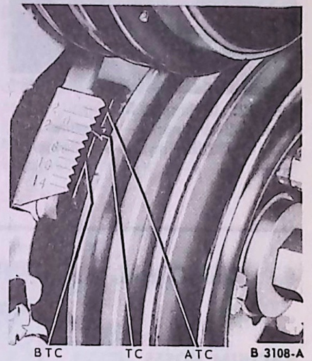
FIG. 20 Typical Engine Timing Marks—Pointer Mounted
