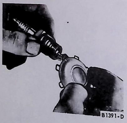
FIG. 27 Checking Spark Plug Gap
