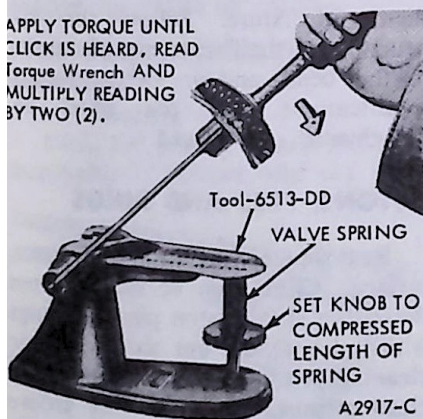
FIG. 36 Checking Valve Spring Pressure
