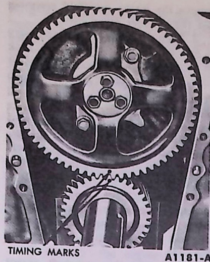
FIG. 15 Timing Mark Alignment
