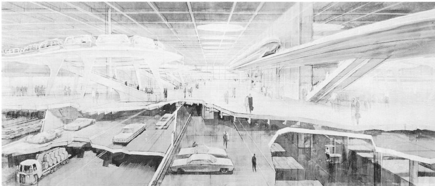
This cutaway rendering shows how differing modes of transportation will be channeled into non-conflicting traffic flows below the pedestrian level of EPCOT. The transportation lobby, shown in the top half of this view, will be located directly beneath the 30-story theme hotel and will be the central arrival-departure point for all passengers using the monorail (upper right) or the newly-designed WEDway PeopleMover (upper left).
