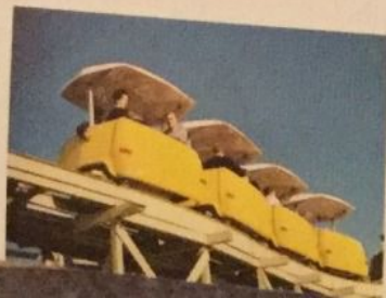
Prototype of the WEDway People Mover system, in operation at WED Enterprises in California. These cars are approximately \frac{1}{4} scale.
