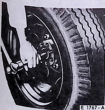
FIG. 141 Axle Shaft Removal Tapered Dowels
