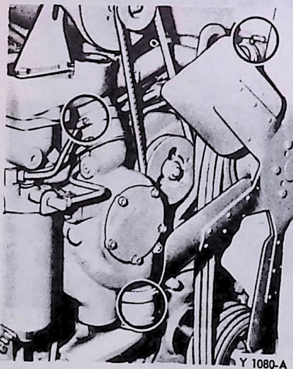
FIG. 94 Cooling System Hoses Check Points
