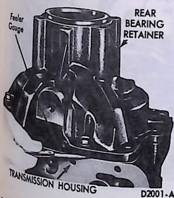
FIG. 61 Rear Bearing Retainer Gasket Measurement
