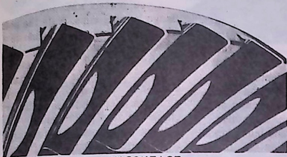
LOW CONTACT THE PINION IS IN TOO FAR. ADD SHIMS, AND READJUST BACKLASH.
