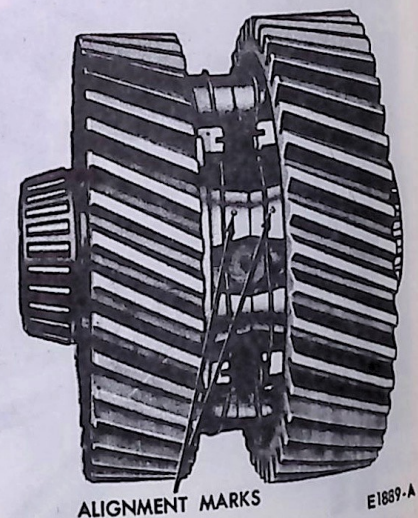
FIG. 35 Differential Case and Gear Alignment Marks
