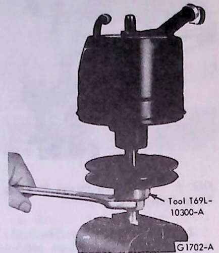
FIG. 5 Removing Power Steering Pump Pulley
