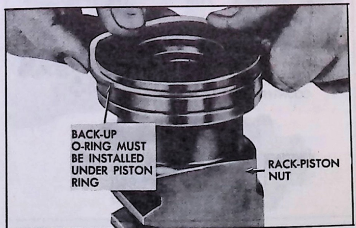
Fig. 47--Installing Ring on Rack-Piston
