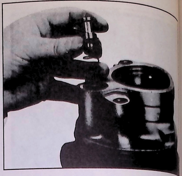
Fig. 30—Installing Flow Control Valve
