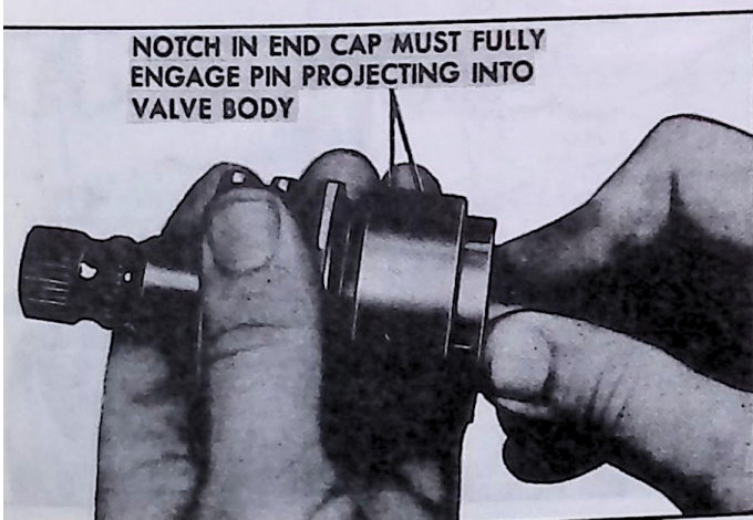
Fig. 46--Installing Stub Shaft Assembly
