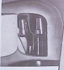
A LUXURY COMPARTMENT is located on either side of the rumble seat. Thermos bottles are of stainless steel . . . glasses of spun aluminum. Compartments light automatically.
