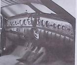
ALL INDICATORS on the instrument panel may be read at a glance. There are fuel, oil, speed, mileage and ampere dials; battery, R.P.M. and engine efficiency indicators; oil temperature and pressure gauges, altimeter. compass, cigar lighters.
