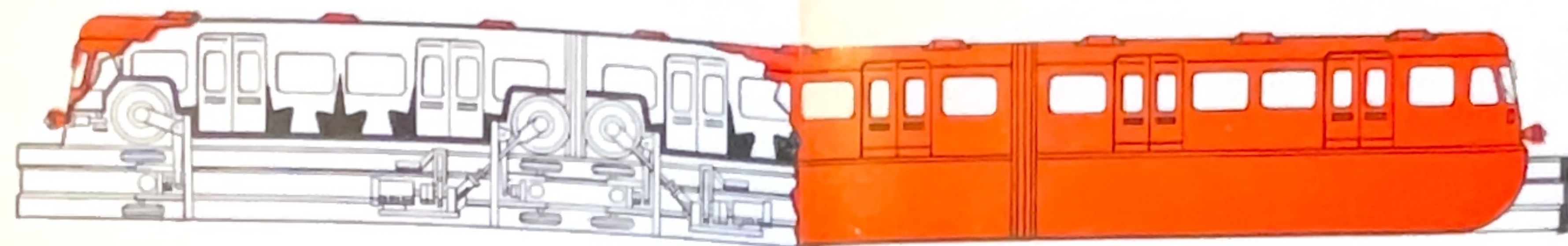
Cutaway showing how Monorail car is built.
